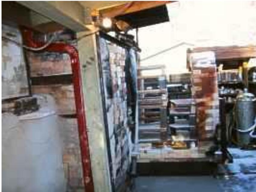
Cart half-way out on old gas and woodfired two-chambered kiln. Note damper for coffin kiln on left. There is a sliding damper that separates the old kiln from the base of the new shared chimney.
