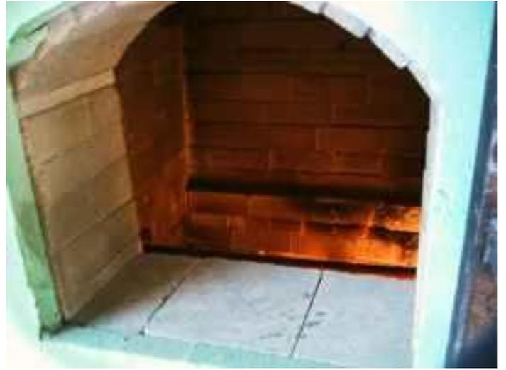
View into lighted firebox with hobs and center rod fire bar.
