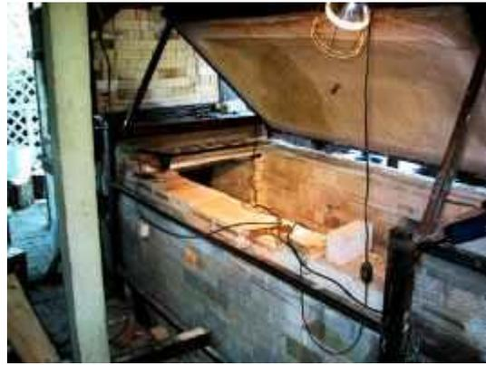
Kiln with lid up and safety bars in place after first test firing, before addition of insulating cast able on wire mesh on exterior. Note kiln shelf top of tumble stack area behind firebox with cast able insulation over silicon carbide shelf
